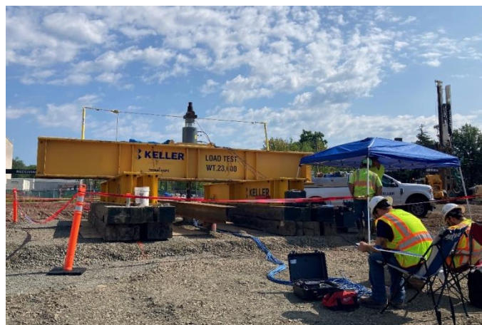
Fig. 1. Micropile Tension Test Setup (Test #1).
