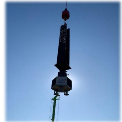
Figure 13 SQUID™ mounted on the Kelly bar (left) and 1 ton beam (right) at the construction site
