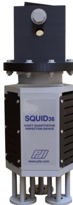
to placement of reinforcement and concrete. To achieve cleaning once drilling is complete, a cleanout bucket is typically used to remove any material unsuitable for end bearing support. Bottom inspection is then performed with SQUID which takes accurate force and displacement measurements, providing an objective, quantitative assessment.
