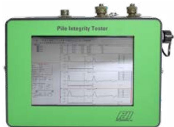
PIT tests may also help estimate the depth of the pile toe (the pile length) if the pile is intact with embedment less than 30 times the pile diameter. PIT data is evaluated in the field and later transferred to a computer for further analysis by the PIT-W software.
