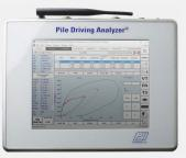
Conforms with ASTM D4945
