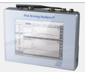
Conforms with ASTM D4945
