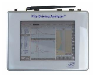
hammer blow the static soil resistance at the time of testing (by Case Method and/or iCAP®, a real-time signal matching analysis), driving hammer performance, maximum driving stresses, and evaluates pile integrity. The high-speed PDA-8G data transmission allows testing at hammer operating blow-rates as high as 120 bpm, without loss of data.
