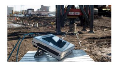
drilled shaft (bored pile) testing. File set-up includes the ability to model force measurements taken on the pile, a load cell, or the ram. Inertial effects are automatically accounted for when testing with the load cell or ram instrumentation.
