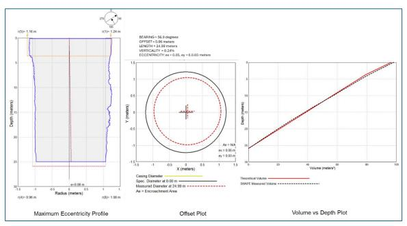
Figure 3. SHAPE profile, offset, and volume vs depth plot for well controlled installation.
