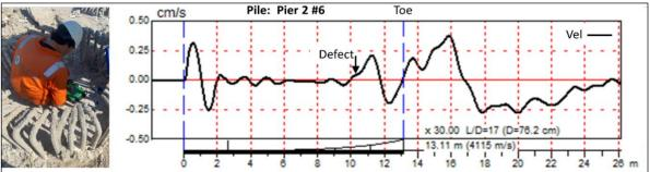
Figure 8. Photo of a PIT test (left) with an example record indicating a defect at 10.2m depth.
