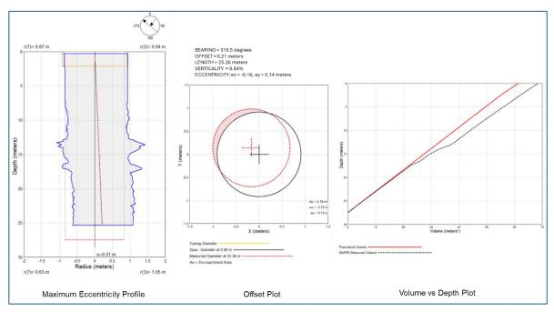
Figure 2. SHAPE profile, offset, and volume vs depth plot in shaft with sidewall instability.
