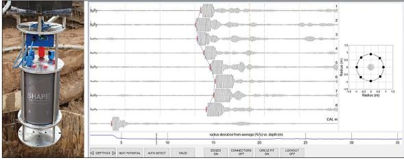
Figure 1. SHAPE device (left) and test results at one test depth from each sensor (right).
