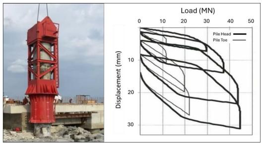
Figure 9. Dynamic load test on bored pile (left) and example test results (right).
