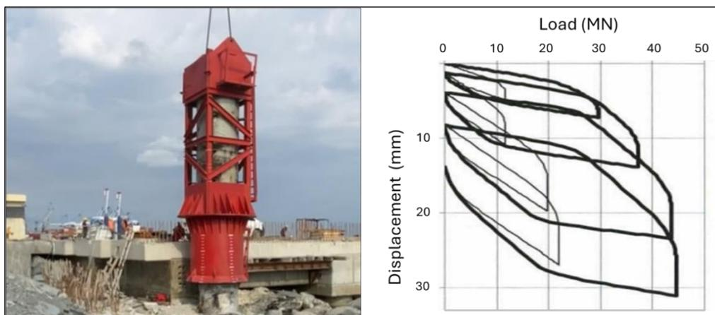
Figure 9. Dynamic load test on bored pile (left) and example test results (right).
