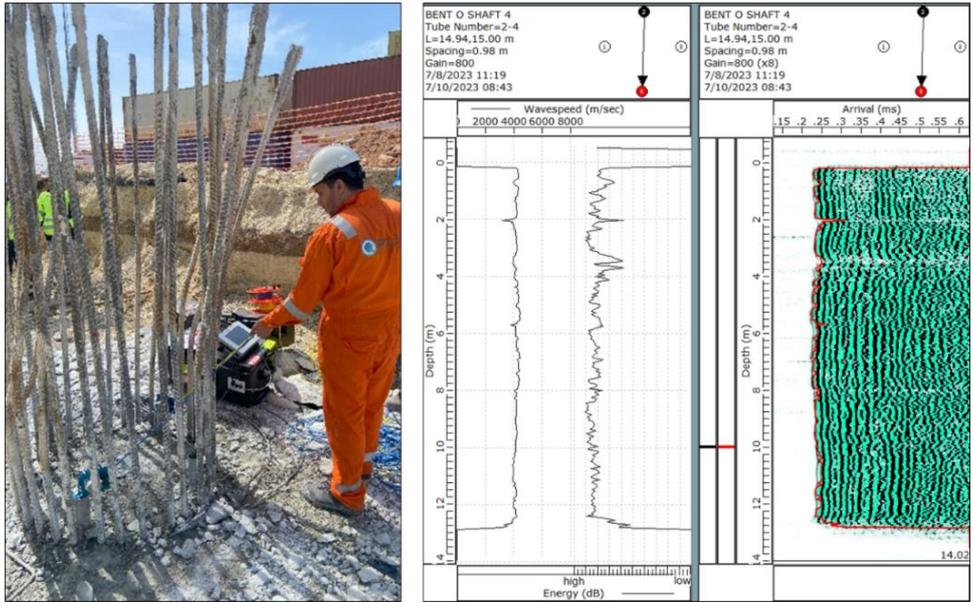
Figure 7. CSL test (left), first arrival time and energy (center) and FAT waterfall (right) vs depth plots.
