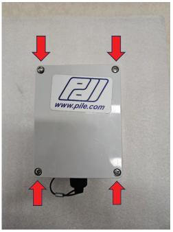
Remove the lid and place it to the side of the device. See the image below.
