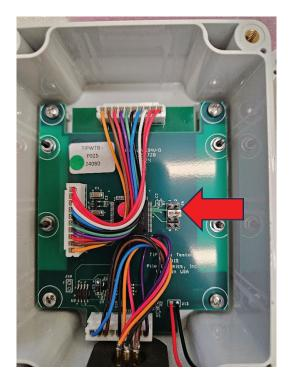
Remove the white jumper from pins 3 & 4 and install in across pins 1 & 2. See the image below.
