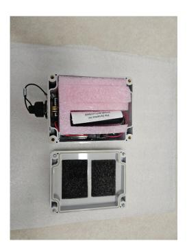
Disconnect the battery pack from the cable assembly and place the entire foam piece outside of the unit. See the image below.
