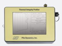
Conforms with ASTM D7949
