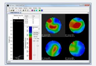
The <u>PIT-Q</u> assesses the structural integrity of drilled shafts/bored piles, ACIP/CFA, and drilled displacement piles, driven concrete or timber piles and concrete filled pipes. The PIT-Q performs wave equation-based, non-destructive foundation investigations known as Low Strain Impact Integrity Tests or Low Strain Dynamic Tests, providing assurance that a pile or shaft is free of major cracks and voids.
