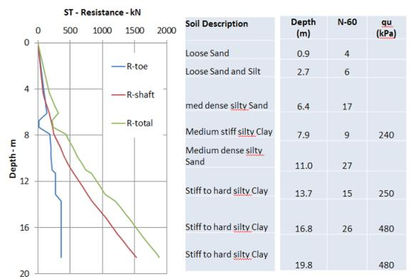
Figure 1. Soil properties and ST pile capacity vs depth.
