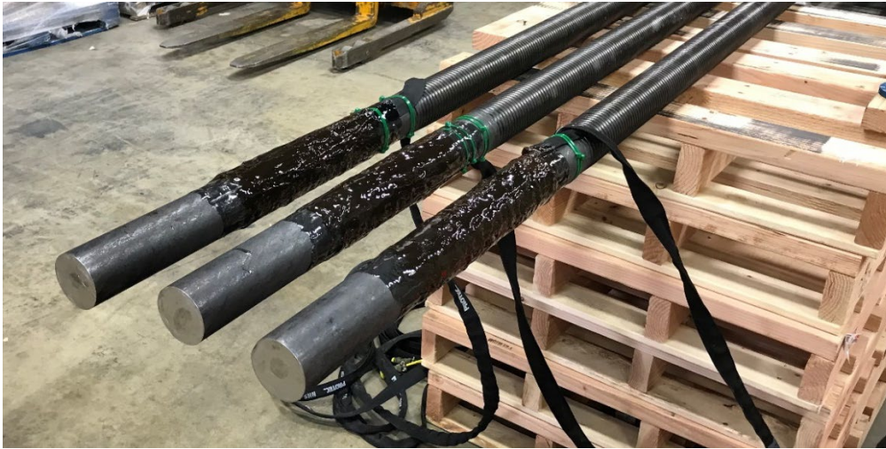
Fig 8. Strain gages attached to 2-foot-long unthreaded portion of TLBT base mobilizer bars
