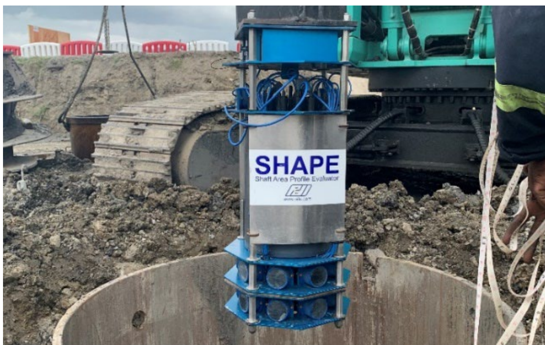
Figure 1. Shaft Area Profile Evaluator being lowered into a bored pile excavation.
