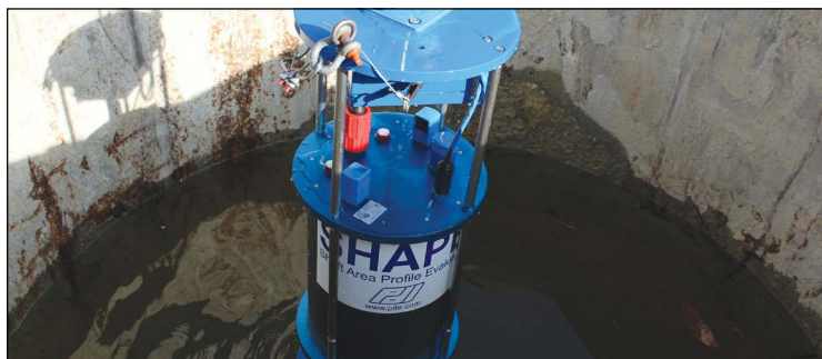
Image 1. Shaft Area Profile Evaluator (SHAPE) descending into drilled shaft
