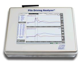
Criterion and contributes to safe and economical production pile installation. The PDA-8G calculates for every hammer blow the static soil resistance at the time of testing (by Case Method and/or iCAP®, a real-time signal matching analysis), driving hammer performance, maximum driving stresses, and evaluates pile integrity. The high-speed PDA-8G data transmission allows testing at hammer operating blow-rates as high as 120 bpm, without loss of data.
