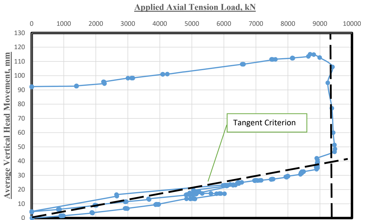
Figure 5: Tension Pile 1 – Load vs. Vertical Movement
