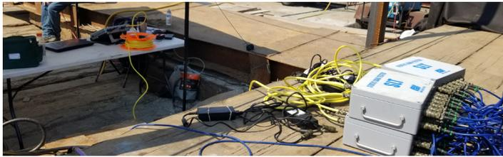
SLT Acquisition Boxes daisy-chained (yellow cables) with smart analog sensors connected (blue cables). The Master Box is connected to a PDI Tablet using the longer yellow Main Cable.
