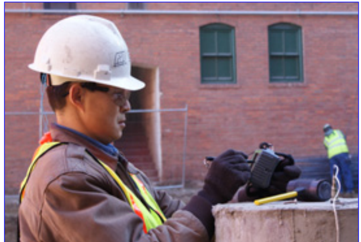
PDI's Dr. Liqun Liang tests an ACIP Pile with PIT-X2 (2 velocity test) in Cleveland, OH
