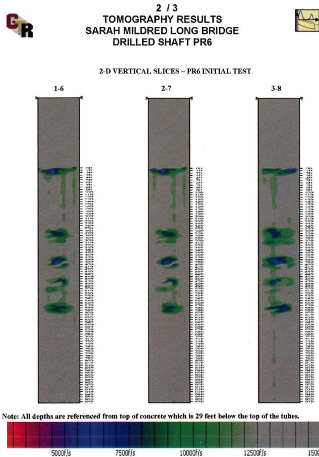
Figure 12: CSL Test Results and Tomography Results (Geosciences Testing and Research, Inc.).
